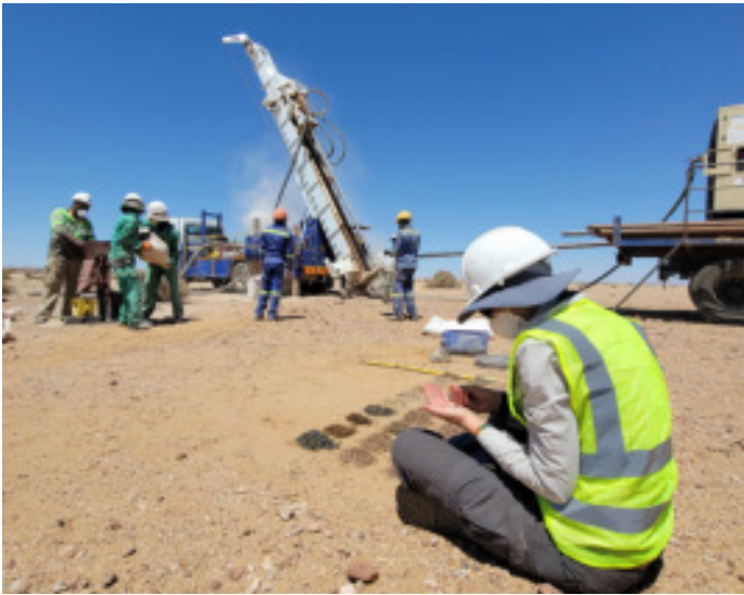
Fig. 2: RC drilling and sampling at the Eureka site
