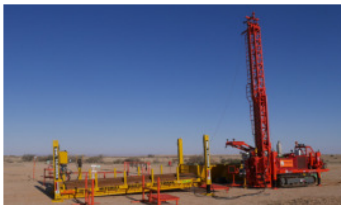
Fig.1: Diamond drilling at the Eureka site
