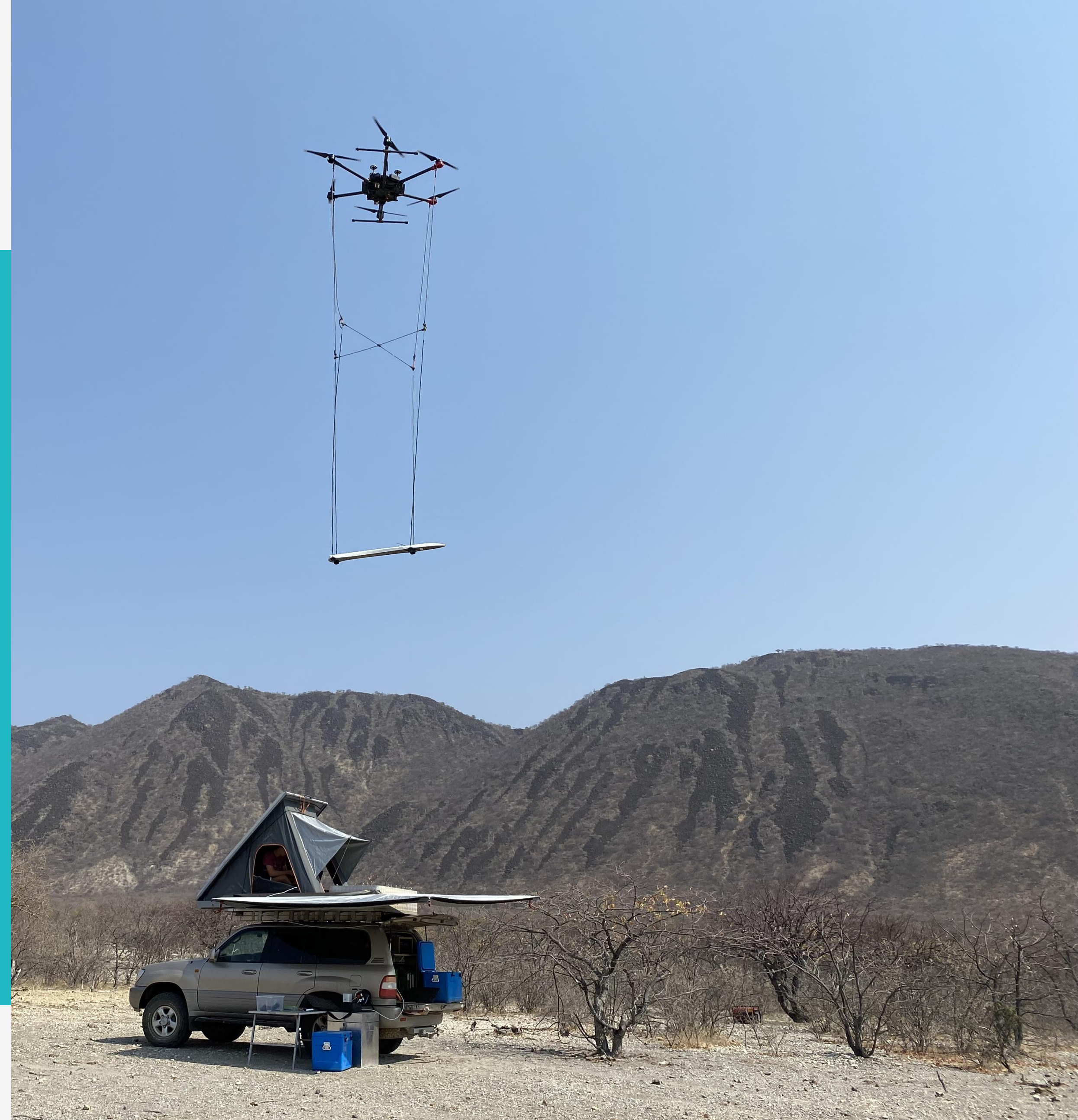
Magnetic sensor suspended beneath the drone
